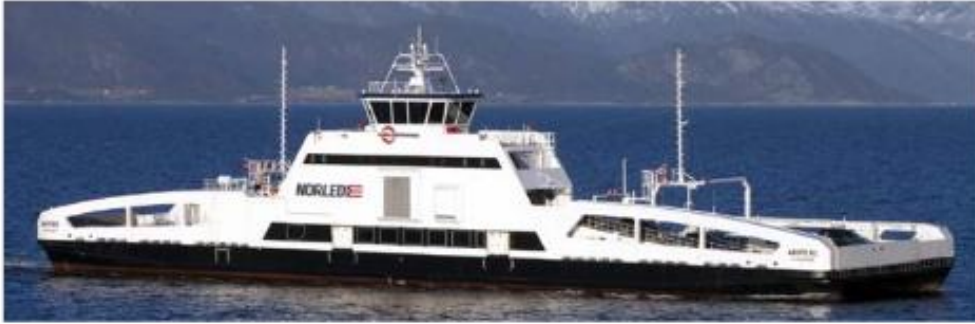
Ampere: battery ferry in operation in Sognefjorden
