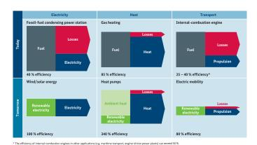
Figure 1: Primary energy consumption (grey and green) versus useful energy services (blue) in today's versus tomorrow's energy system. (Reproduced with permission from [93], page 86; based on [94])
